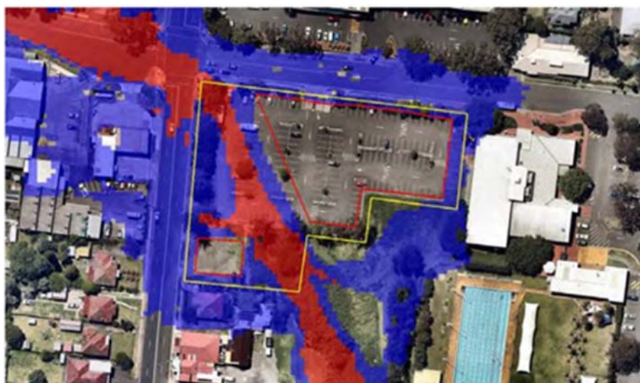
Figure 6.1-2 1% AEP Post-Development Provisional Hydraulic Hazard
